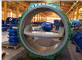
Fig. 1- DN 1800/PN 10 Butterfly Valve
