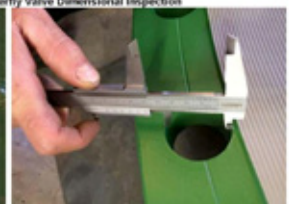
Fig. 11 & 12- DN 1800/PN 10 Butterfly Valve Dimensional Inspection
