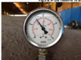
Fig. 5- Pressure Gage showing Test Pressure
