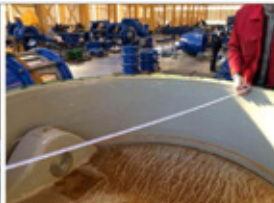
Fig. 13 & 14- DN 1800/PN 10 Butterfly Valve Dimensional Inspection
