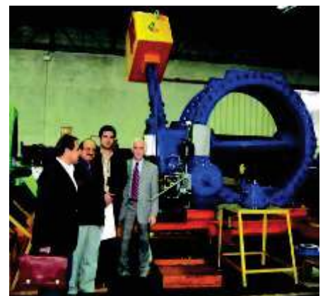
Normally open (fail to close) emergency Excess shut off valve DN1800, PN25 IDOGHMOUSH Dam, IRAN.
