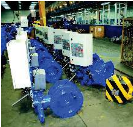
Normally open (fail to close) emergency Excess shut-off valve DN350, PN16 Water supply project in ZAHAK (Water & WasteWater of Systan & Balouchestan, IRAN),
